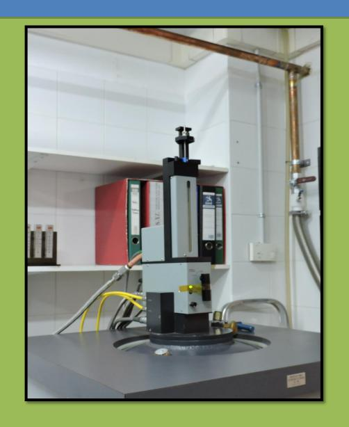
This technique let us study the magnetic properties of the material by creating an intense magnetic field with the help of a superconducting coil.
